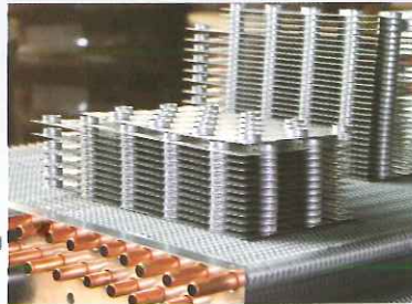
Geometry 32.0x27.7 mm for pipes \varnothing 12 \times 0.4
